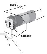
The motor cable should not act as a direct conduit for the water to enter the head of the motor (form drip loops).
