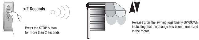
e) The new DOWN or extended limit has been recorded. Repeat the same procedure for the UP or retracted limit.
