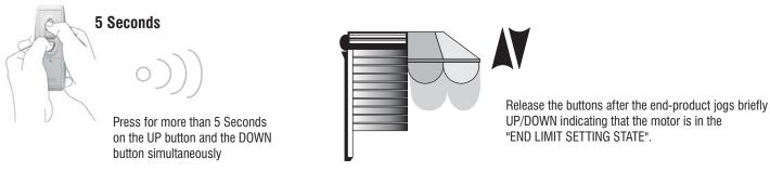
c) Adjust the DOWN limit to the new position (the motor will respond to the transmitter in a momentary fashion).d) Record the new DOWN limit.
