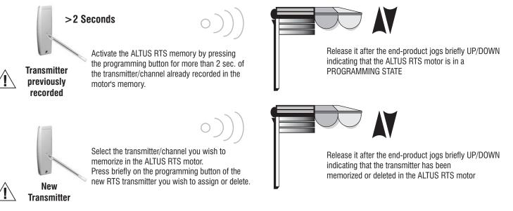
Repeat this procedure for each additional transmitter/channel you wish to add or delete. It is not possible to delete the transmitter/channel used to enter the programming state.
