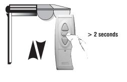
If necessary adjust the correct UP position by using the UP and DOWN buttons. Record the UP and DOWN positions by pressing the STOP button for more than 2 seconds. The setting of the end limits is now completed.
